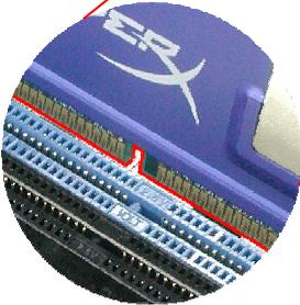
**Note:** The tabs of the DIMM slot will clip to hold the DIMM in place when the DIMM touches the slot's bottom.
